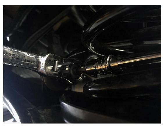
**Step 3** – Assemble each 034Motorsport MQB Audi/Volkswagen Spherical Rear Sway Bar End Link with two large spacers (402-Z011) at the bottom and one small spacer (402-Z010) at the top.
