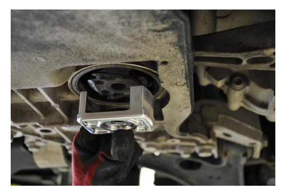
**Step 4** – Reinstall the factory dogbone mount bolt. Torque to 100 Nm + 90 Degrees.
