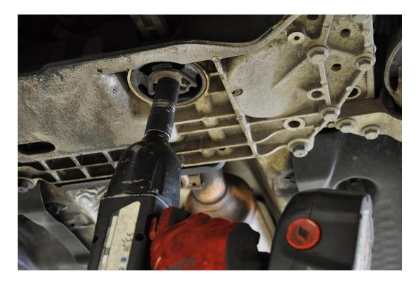
**Step 3** – With the factory bolt removed, you can install the Billet Aluminum Dobgone Mount Insert into the voids. It should be positioned with the 034Motorsport logo towards the front of the car.
